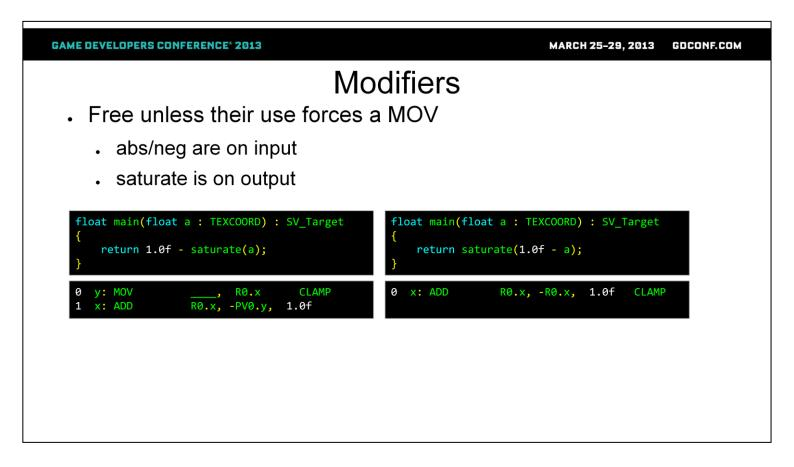
saturate() on the other hand is on output. So you should avoid calling it directly on any of your inputs (interpolators, constants, texture fetch results etc.), but instead try to roll any other math you need to do on it inside the saturate() call. This is not always possible, but prefer this whenever it works.
