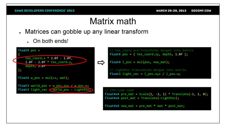
Here we are converting a screen-space texture coordinate and depth value into a world-space coordinate, which is then used for computing a light vector. These transforms can be merged into the same matrix. Naturally chained matrix transforms can also be merged into the same matrix. We have had real shaders where merging the transforms ended up more than doubling the performance.
