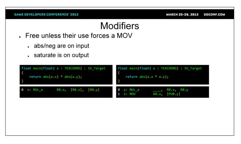
You want to place abs() such that they happen on input to an operation rather than on output. If abs() is on output another operation has follow it for it to happen. If more stuff happens with the value before it gets returned, the abs() can be rolled into the next operation as an input modifier there. However, if no more operations are done on it, the compiler is forced to insert a MOV instruction.
