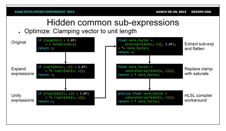
The most obvious optimization, i.e. removing the sqrt() call and comparing the length squared instead, is a bit of a dead-end. We get further by unifying the expressions instead. Once the expressions are unified, we can pull out the normalizing factor, and then simply flatten the if-statement though clamping the factor to 1.0f. As we don't expect any negative numbers, this clamp can be replaced with saturate(). Finally, HLSL realizes as much too, so we need to apply the precise workaround.
