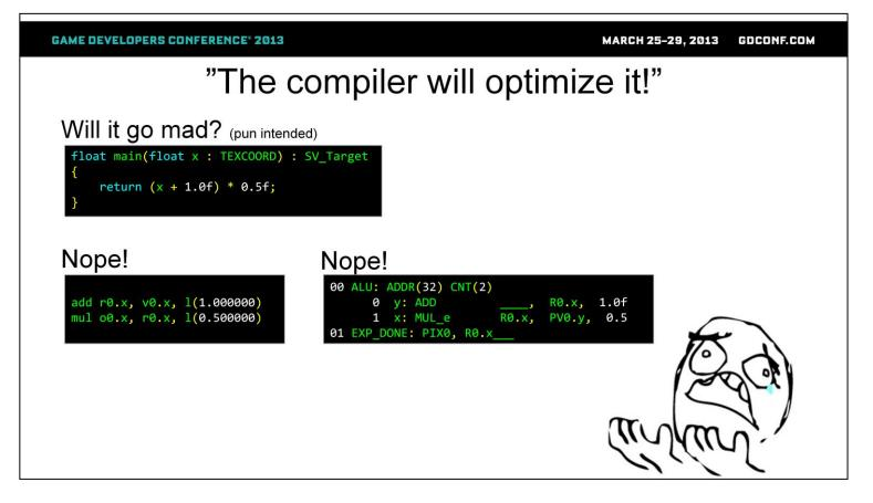
The driver is bound by the semantics of the provided D3D byte-code. Final code for the GPU is exactly what was written in the shader.
